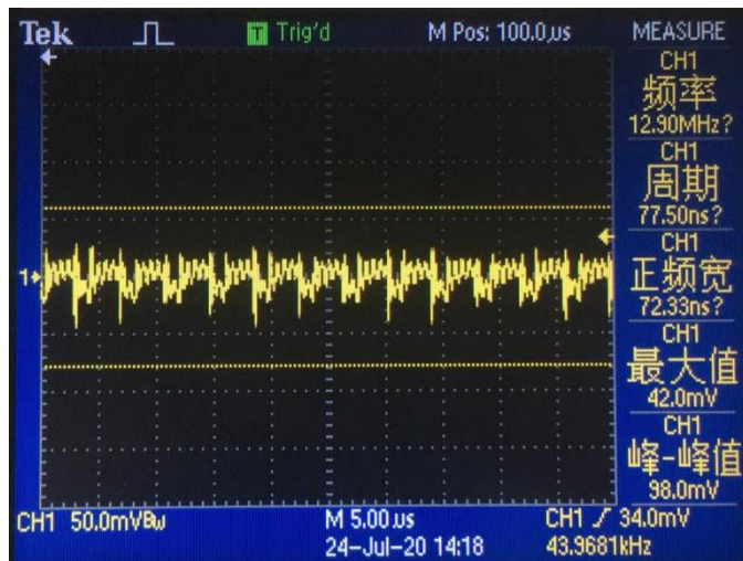
Noise (VIN = 48V, IO = 1.1A, 5 ~ 20MHz bandwidth)
